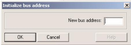
If **only one** transmitter is connected to the software, the bus address of this transmitter can be changed via the **Init bus address of instrument** button. Enter the new bus address in the message (e.g. 009) and click on **OK** to confirm.
